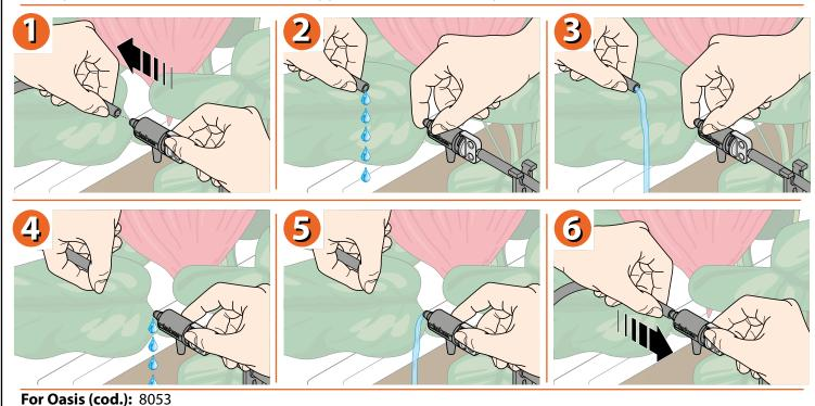
Cleaning the filter. The filter must only be removed and refitted when the tank is empty.
