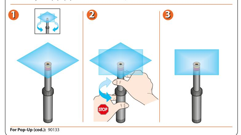
**ADJUSTING THE RANGE.** To increase or reduce the length of the jet, just a few simple steps are required. Using a 3mm hex socket key, turn the internal adjuster screw anticlockwise for a longer jet, or clockwise for a shorter one.
