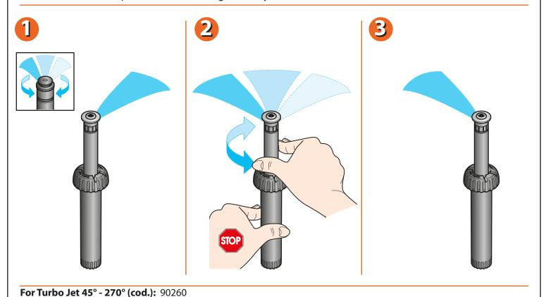
**ADJUSTMENT OF SPRAY ANGLE BETWEEN 45° AND 270°.** This adjustment serves to increase or reduce the coverage of the sprinkler. Using the key provided, turn the collar located under the sprinkler head, which is marked with symbols for adjustment purposes. To select the required working angle, hold the sprinkler head (marked with the symbol "R") and the stem fast, and turn the collar anticlockwise to increase the coverage, or clockwise to reduce it.
