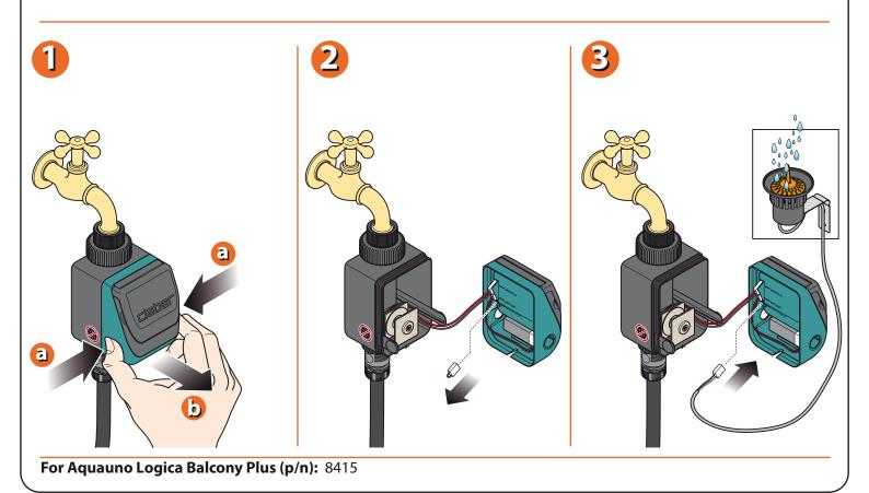
At the end of the warm season and before the first winter frosts, disconnect the timer from the tap and store it indoors, bearing in mind to remove the battery.
