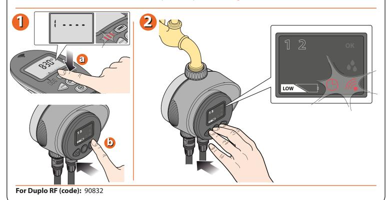
While the timer display keeps blinking, press the hidden button on the radio remote control with the tip of a paper clip. The display will start to blink and the symbol will appear. The connection will be successfully completed when the message appears on the remote control and the timer starts an initialization cycle (Leds light up in sequence, valves close in sequence).
