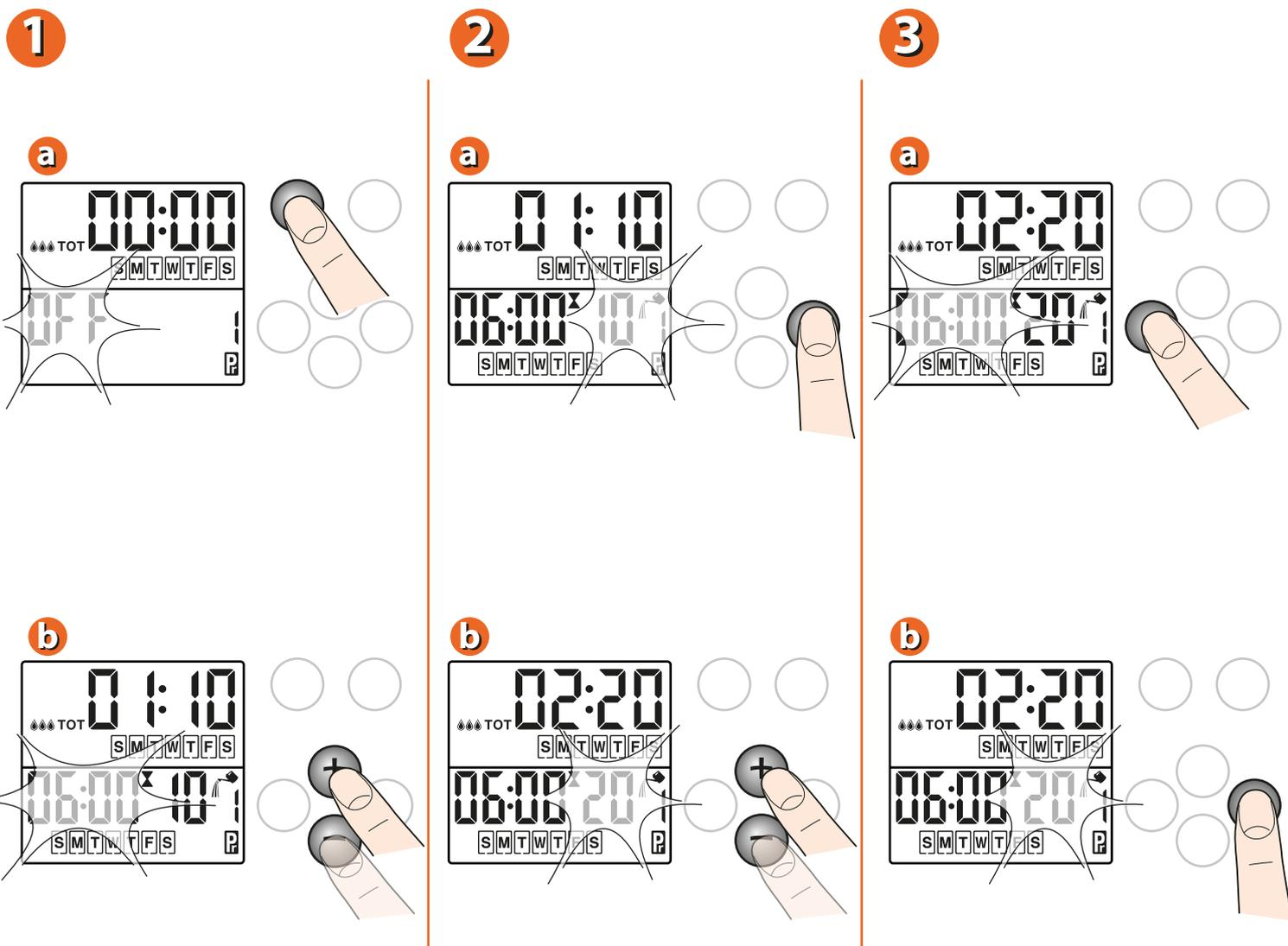
**PROGRAMMING WATERING - Watering days (1-2).** If the PLUS FUNCTION has been previously set to Off, after having set the watering run time, press A to access the settings for the Days of the week on which each programme is to be carried out 1... 4.
