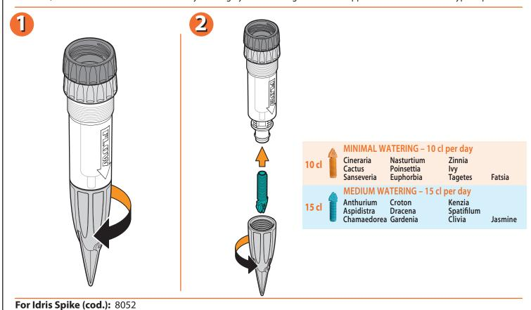
Fill the plastic bottle with water. Select the adapter compatible with the thread of the bottle. Screw the IDRIS tripod onto the bottle.
